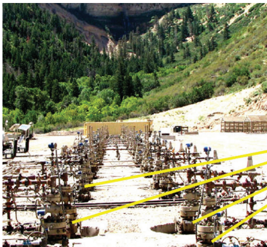
Fig. 12. Drilling of wells from one site (Colorado, USA). The arrows show wells drill in a single pad by the same drill rig
